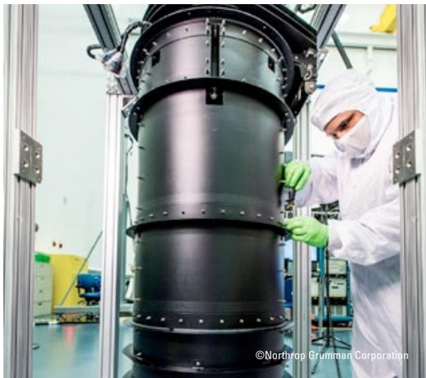
Once in space, the DTA extends 1.5 meters and lifts over 3,311 kilograms (7,300 lbs.), to deploy the primary mirror, secondary mirror array, and backplane equipment.
