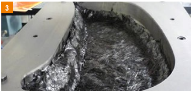
3 The preform is transferred to the cavity of the preheated compression molding tool.
