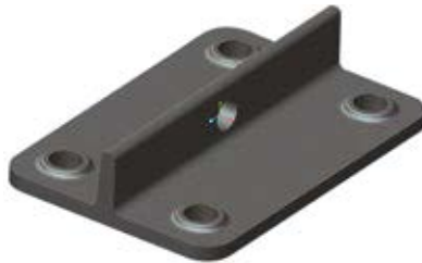
Figure 2. Replicates the design with composites, molded thicker overall at the same weight, added support near holes, and rounded edges.
