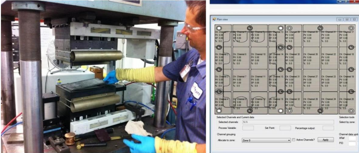
Figure 7. XPress tooling setup and heating zones.
