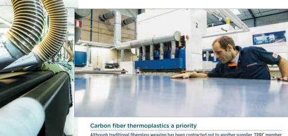
Although traditional fiberglass weaving has been contracted out to another supplier, TPRC member TenCate's Nijverdal plant continues to weave carbon-fiber fabrics, which are eventually prepregged with thermoplastic resin at the facility to become CETEX thermoplastic sheet products, in one of three large presses. Source (both photos) | TenCate/© TenCate
