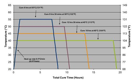
Alternative cure cycles at higher temperature may be used e.g., 4 hours at 60°C (140°F) Caution: Toray AmberTool® HX56 prepreg contains a reactive resin system and care must be taken to avoid exothermic heating during the initial cure. Avoid exceeding 65°C (149°F) during the initial cure.
