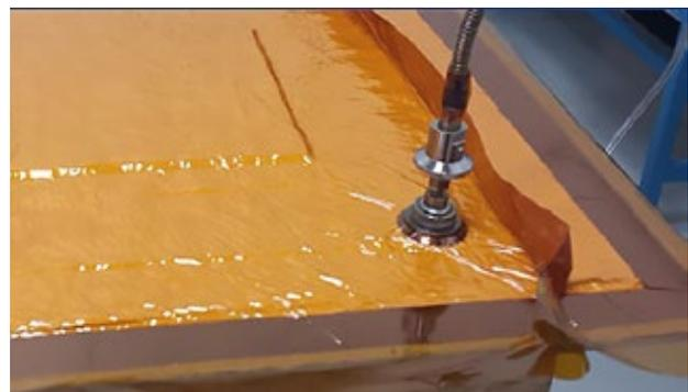
*Figure 3. State of art. Toray Cetex® TC1225 looks good—results in a fast vacuum-aided oven consolidation process*
