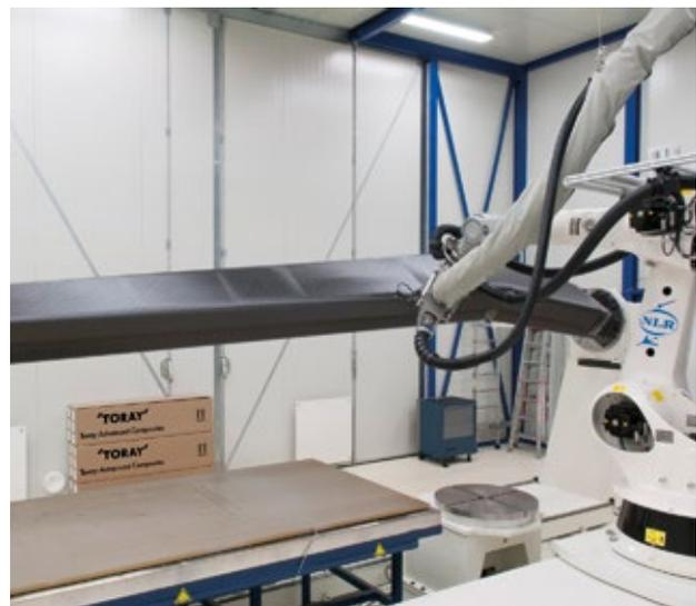
*Figure 4. Nearing the ultimate goal: Toray Cetex® TC1225 looks promising—results for full in situ tape placement*
