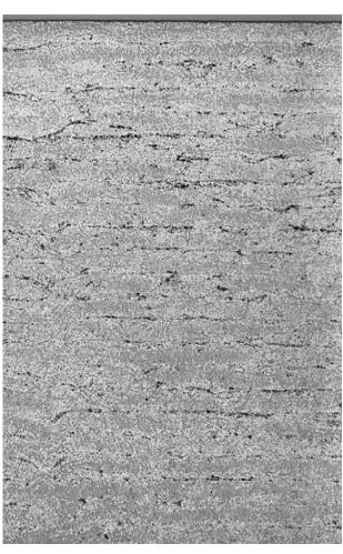
Figure 6. Micrograph after in situ tape placement at deposition rates >200mm/s
