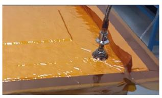
Figure 3. State of art. Toray Cetex® TC1225 looks good—results in a fast vacuum-aided oven consolidation process
