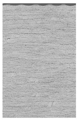
Figure 5. Micrograph after tape placement and oven consolidation
