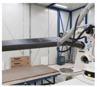
Figure 4. Nearing the ultimate goal: Toray Cetex® TC1225 looks promising—results for full in situ tape placement
