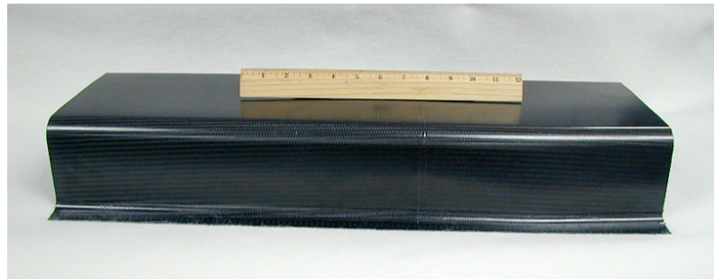
Demonstration part of 100+ plies of TC275-1, with less than 1% voids.
