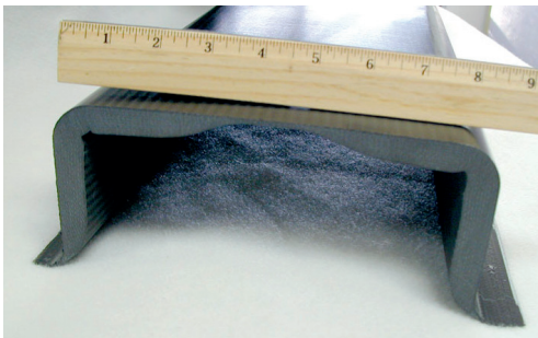
Demonstration part of 100+ plies of TC275-1, with less than 1% voids.
