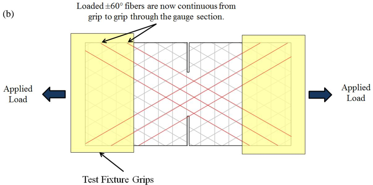
Figure 1. (a) Demonstration of the inadequacies of the ASTM 3039 straight sided coupon for tensile testing of braided composites in the  $90^\circ$  direction. (b) The notched coupon developed to give accurate strength measurements of braided composites in the  $90^\circ$  direction.
