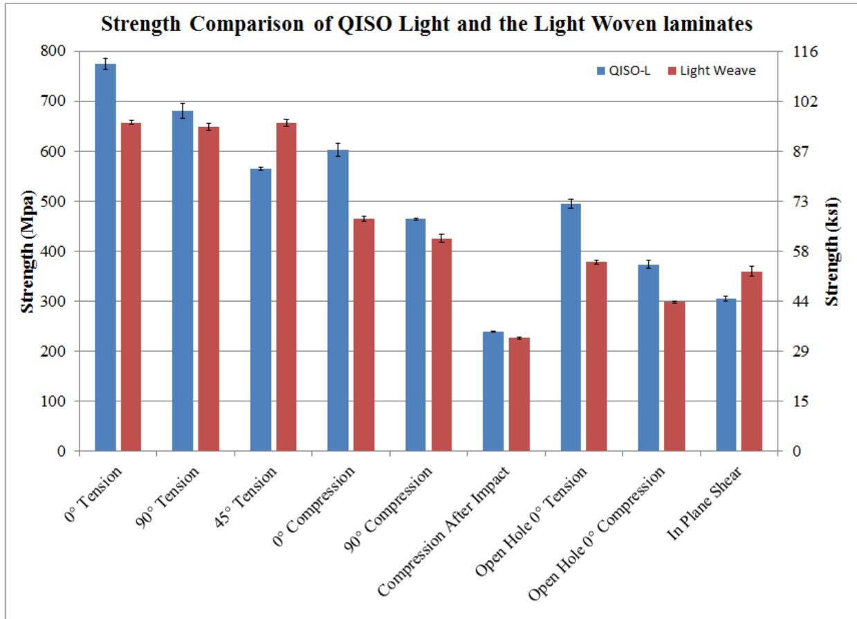
Figure 3. Graphical representation of strength data comparing the QISO Light laminate and the Light Woven laminate.
