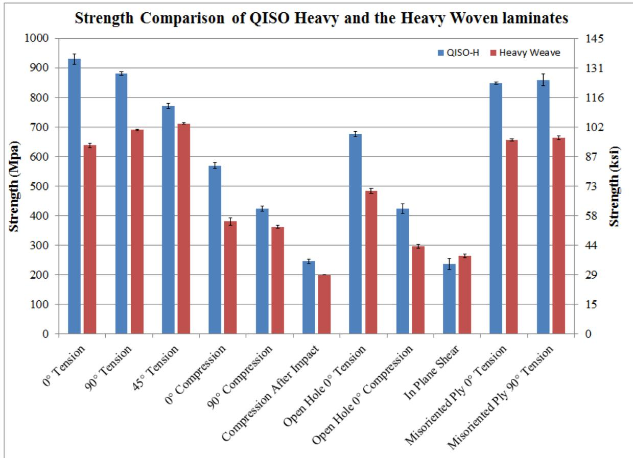
Figure 2. Graphical representation of strength data comparing the QISO Heavy laminate to the Heavy Woven laminate.
