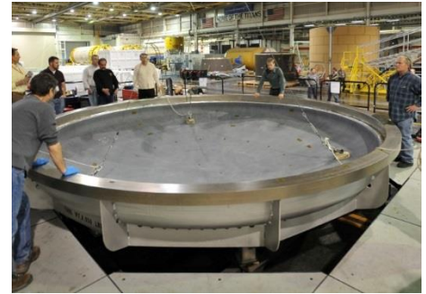
Lockheed Martin Denver Orion Heat Shield utilizes TenCate prepregs in a low pressure out of autoclave cure process.
