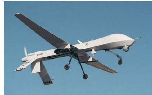
General Atomics Aeronautical Systems utilizes prepregs from TenCate in low pressure curing processes for Reaper and Predator programs.
