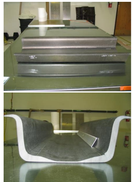
Demonstration parts fabricated both in autoclave and out of autoclave to confirm processing equivalency.
