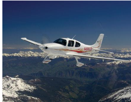
The highly popular Cirrus SR-22 series of aircraft features both fuselage and wing structure manufactured in out of autoclave vacuum cure pressure conditions.
