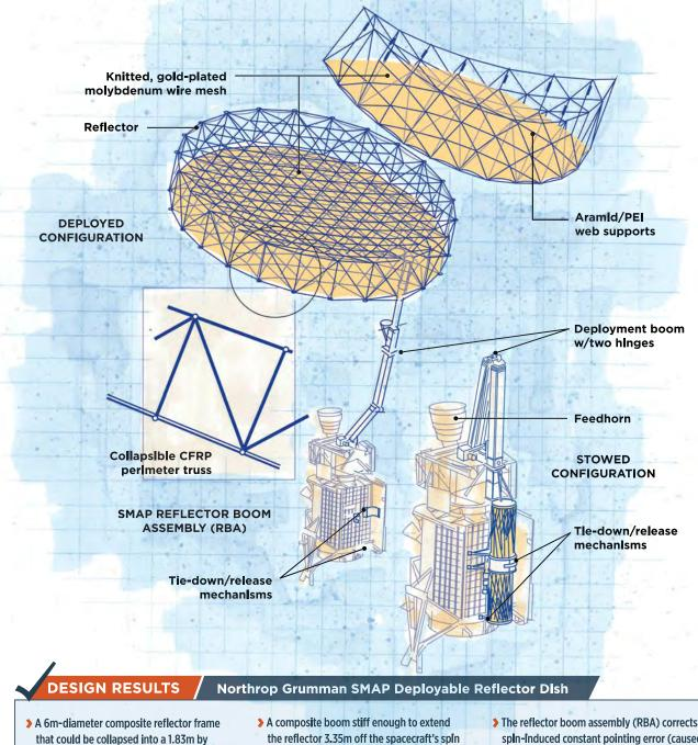
that could be collapsed into a 1.85m by 0.36m envelope for launch, weigh less than 13 kg and then deploy as expected in the zero-gravity LEO environment. A composite boom stiff enough to extend the reflector 3.35m off the spacecraft's spln deck at a 40° angle and to hold the antenna in expected alignment without distortion at 14.6-rpm rotation speeds.
