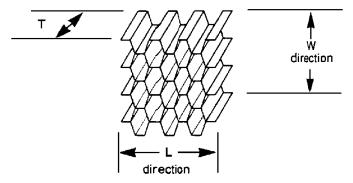
T = Thickness or cell depth L = Ribbon direction W = Direction perpendicular to the ribbon direction
