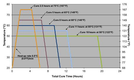
$\label{eq:caution:Toray} \mbox{AmberTool}^{\circledast}\mbox{HX42 prepreg contains a reactive resin system and care must be taken to avoid exothermic heating during the initial cure.}$
