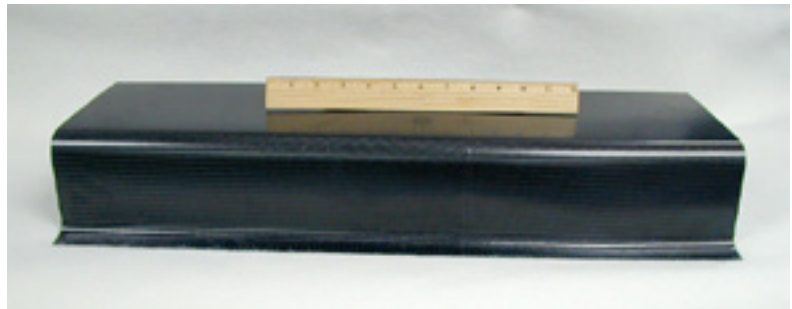
Demonstration part of 100+ plies of TC275-1E, with less than 1% voids.
