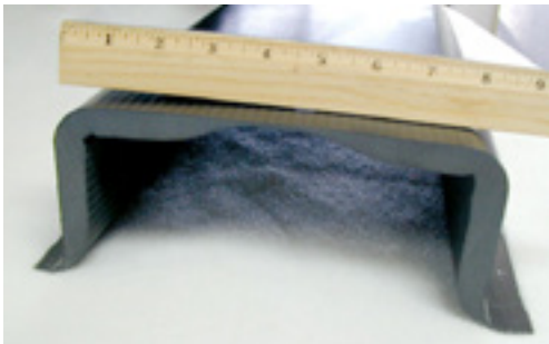
Demonstration part of 100+ plies of TC275-1E, with less than 1% voids.
